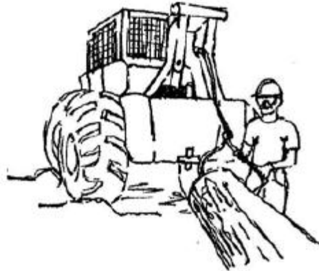
Figure 46 — Hookers shall wear safety gloves when handling cable (Source: Southwide Safety Committee. 1995)
