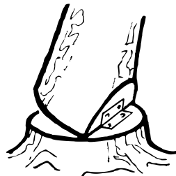
Figure 21 — The hinge is key to steering the tree in the chosen direction (Source: Skogsarbeten (Forest Operations Institute of Sweden) 1984)
