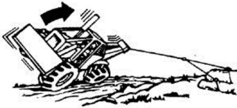
Figure 47 — Do not winch at severe angles to avoid rollover (Source: Southwide Safety Committee. 1995)
