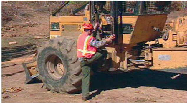
Figure 44 — Nearly one-half of the injuries suffered by equipment operators result from slipping and falling while getting on or off the machine or while working on the machine (Source: Virginian Cooperative Extension 2009)
