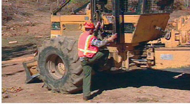
Figure 60 — Nearly one-half of the injuries suffered by equipment operators result from slipping and falling while getting on or off the machine or while working on the machine (Source: Virginian Cooperative Extension 2009)
