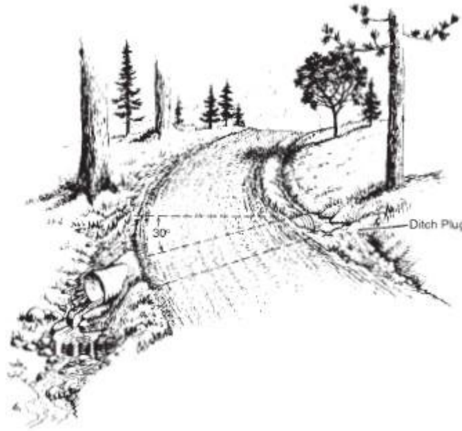
Figure 27 — Install culverts at a 30-degree angle and protect outfall (Source Oklahoma State University 1991)
