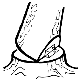
Figure 36 — The hinge is key to steering the tree in the chosen direction (Source: Skogsarbeten (Forest Operations Institute of Sweden) 1984)
