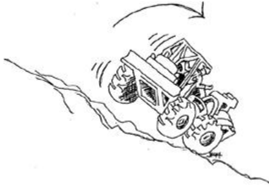
Figure 64 — Never skid across the slope to avoid rollover (Source: Southwide Safety Committee. 1995)
