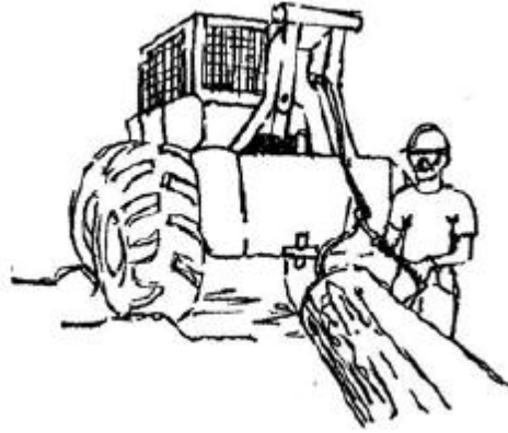
Figure 62 — Hookers shall wear safety gloves when handling cable (Source: Southwide Safety Committee. 1995)
