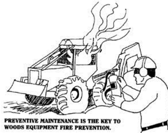
Figure 53 — Proper portable fire suppression equipment shall be located on each unit of mobile equipment (Source: National Timber Harvesting and Transportation Safety Foundation 1995)
