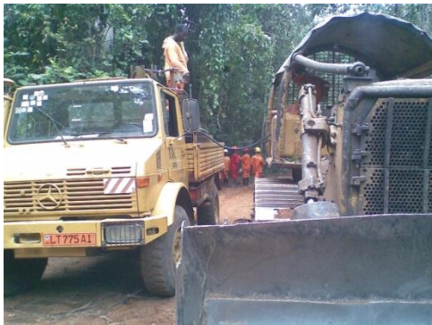
Figure 47 — Suitable equipment should be used for the refuelling of vehicles and machinery (Photograph P. van der Hout)
