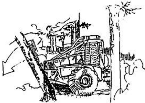
Figure 58 — Lodged trees should be pulled or pushed down with the aid of a skidder
