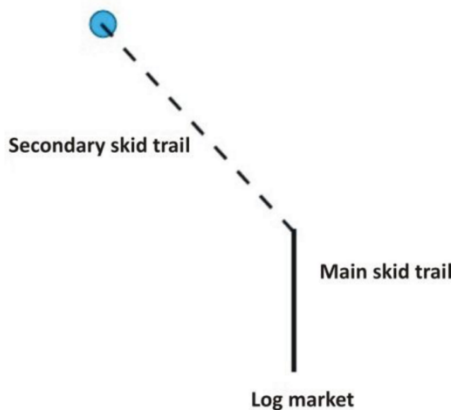
Figure 8 — Branch trail at the end of a skid trail at an angle of 45 degrees (Forêt Ressources Management 2005)
