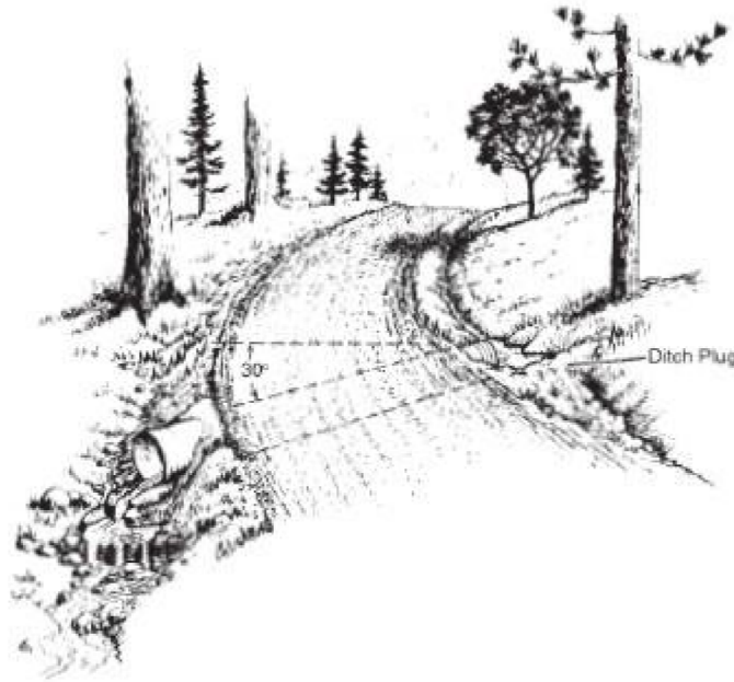
Figure 27 — Install culverts at a 30-degree angle and protect outfall (Oklahoma State University 1991)
