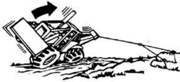
Figure 63 — Do not winch at severe angles to avoid rollover
