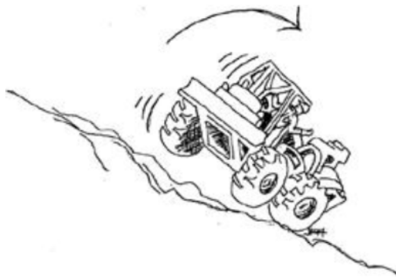
Figure 64 — Never skid across the slope to avoid rollover
