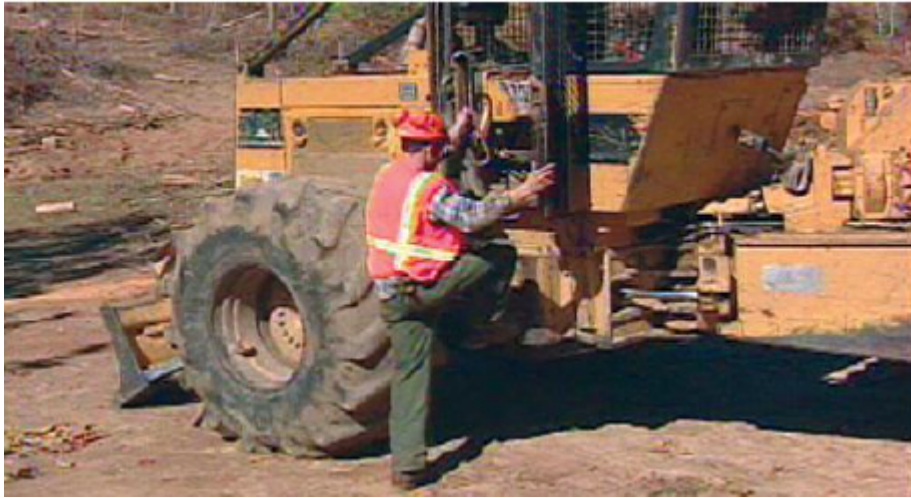
Figure 60 — Nearly one-half of the injuries suffered by equipment operators result from slipping and falling while getting on or off the machine or while working on the machine.
