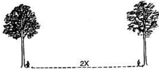
Figure 57 —Workers shall be at least a 2 tree-length away from the tree being felled.
