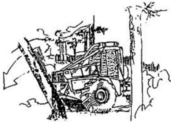
Figure 42 — Lodged trees should be pulled or pushed down with the aid of a skidder (National Timber Harvesting and Transportation Safety Foundation 1995)
