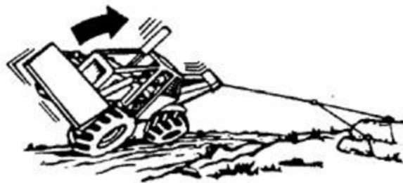
Figure 47 — Do not winch at severe angles to avoid rollover (Southwide Safety Committee 1995)
