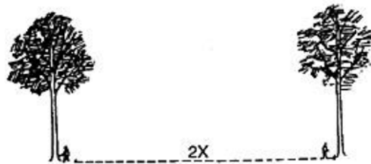
Figure 41 —Workers shall be at least a 2 tree-length away from the tree being felled (National Timber Harvesting and Transportation Safety Foundation 1995)
