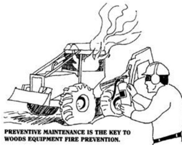
Figure 37 — Proper portable fire suppression equipment shall be located on each unit of mobile Equipment (National Timber Harvesting and Transportation Safety Foundation 1995)
