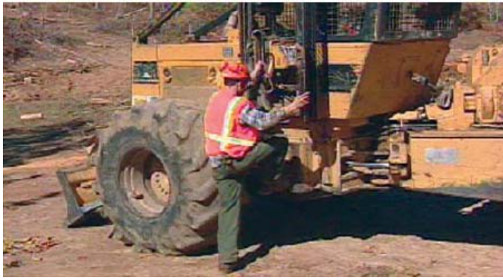
Figure 44 — Nearly one-half of the injuries suffered by equipment operators result from slipping and falling while getting on or off the machine or while working on the machine (Virginian Cooperative Extension 2009)
