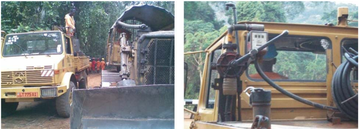
Figure 31 — Suitable equipment should be used for the refuelling of vehicles and machinery (Photograph P. van der Hout)
