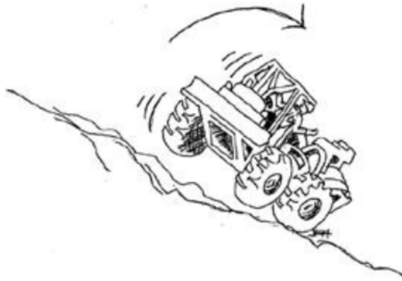
Figure 48 — Never skid across the slope to avoid rollover (Southwide Safety Committee 1995)
