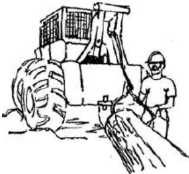
Figure 46 — Hookers shall wear safety gloves when handling cable (Southwide Safety Committee 1995)
