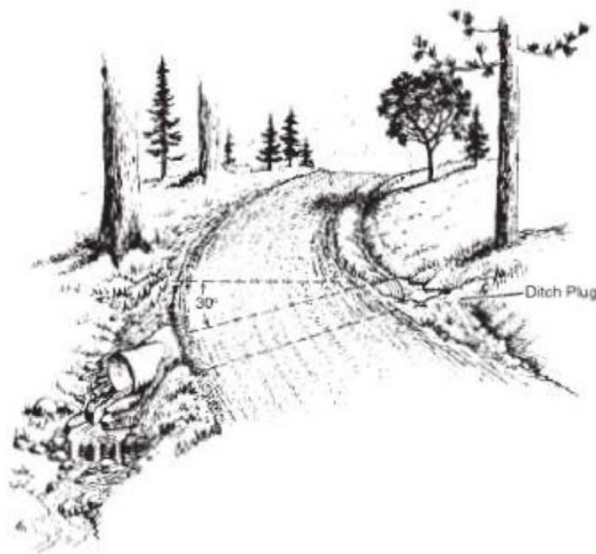
Figure 13 — Install culverts at a 30-degree angle and protect outfall (Oklahoma State University 1991)
