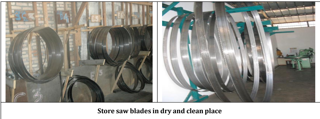
Figure 21: Storage of blades
