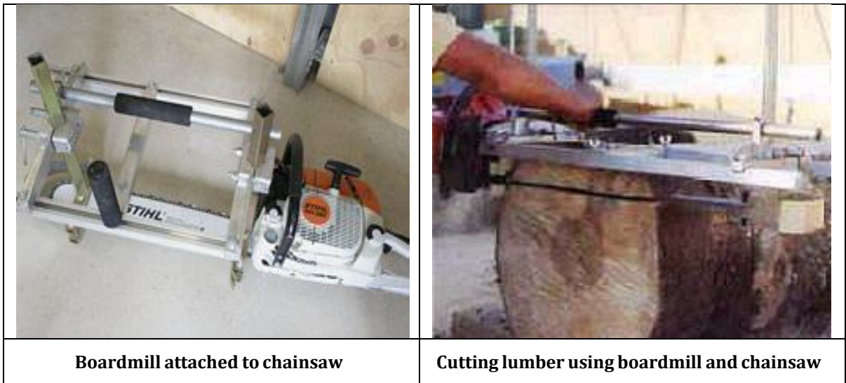
Figure 20: Use of Boardmill with chainsaw for processing logs
