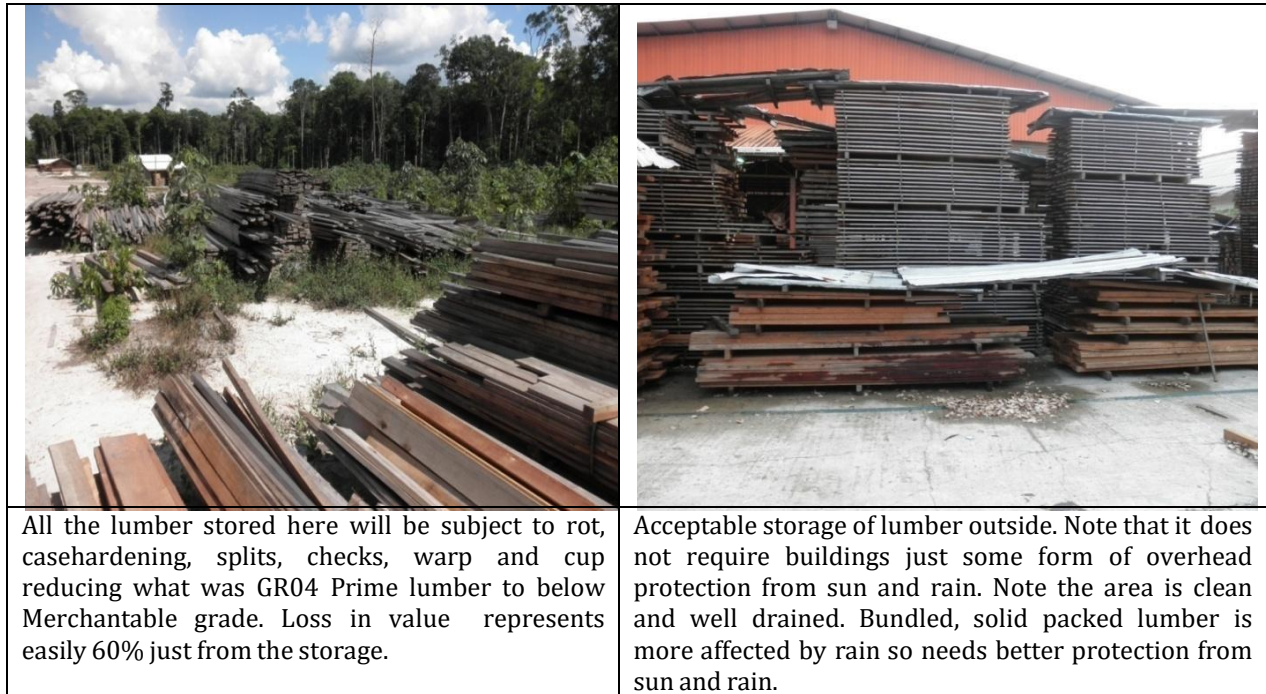
Figure 24: Proper and improper storage of lumber
